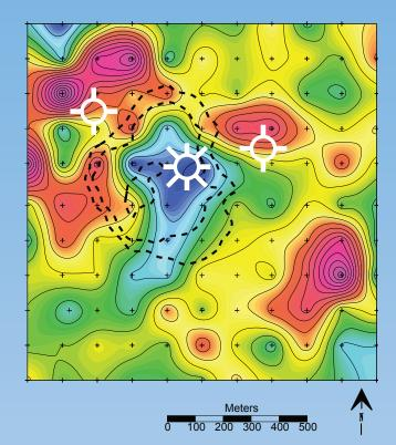
Combined factor plot of *Enzyme Leach*<sup>SM</sup> data with superimposed 3D seismic time structure contours above the Bromhead oil pool at a depth of 2850 m.
